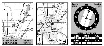
The 30-mile zoom figure (left) clearly shows the dotted course line connecting your current position to your destination. The 30-mile zoom (center) shows both current position and direction to destination on screen. The Navigation Page (right) will also show parigation information
